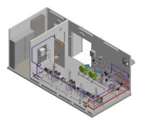
**Cooling Tower Water Treatment Building** Fiberglass shelter with multiple chemical feed systems and separate control room for electrical equipment.
